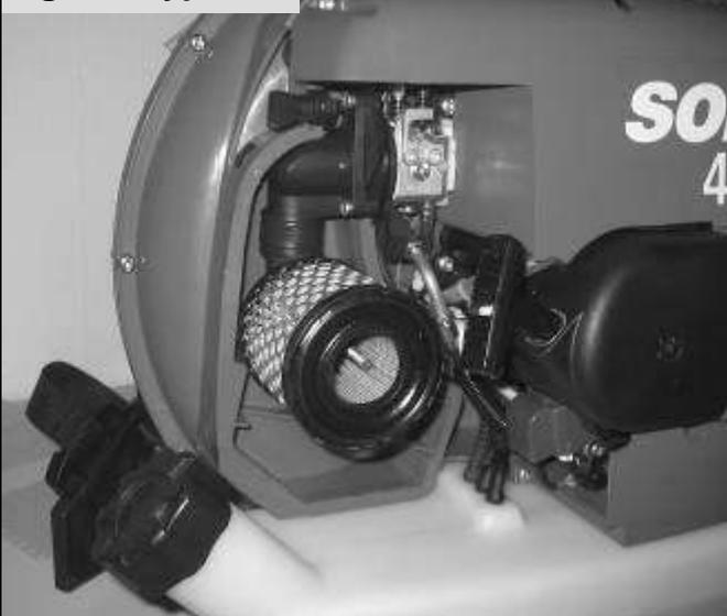
Undo the screw (Fig. 1, Pos 8) completely (screw is retained inside the filter cover) and remove the filter cover.
