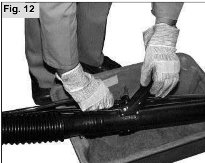
Above the container, pull the supply hose from the shut-off valve.
