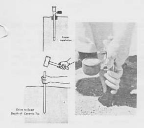
Drive a hole in the ground with an IRROMETER Installing Tool or with a standard piece of ½" Pipe. Standard ½" pipe will make a hole for an exact fit. Install in the root zone of the crop. Insert IRROMETERS in the hole, leaving at least 1" of space between the bottom of the gauge and ground surface. Be sure instrument is "seated" firmly in the bottom of the hole.
