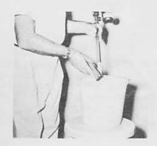
In seasonal cropping, where the ground will lie fallow over the winter, remove IRROMETERS before the first frost, clean exterior thoroughly with water. DO NOT let the ceramic tip dry while dirty. Soak the tip in a clean plastic bucket of water over night with clean water draining through the tip, gravity flow. Air dry instruments and store. Gauges may have water in them and must be stored where temperatures are above freezing.
