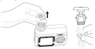
Activate the **MANUAL** mode by pressing the **MANUAL** button. Open the valve and spray water through the valve and the faucet connection to flush out any built-up sediments or debris.
