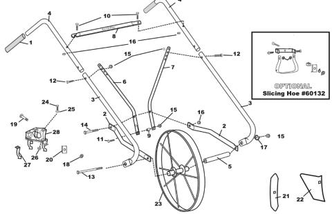
through both (#6 & #7) Tool Supports, then through (2) Frame on the other side and secure with (#16) lock nut, and tighten.
