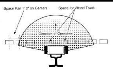
Once the pattern is uniform, the effective pattern width can be determined. The effective pattern width is the distance out from the spreader to a point where the amount of material is 1/2 the average amount in the center pans. This distance is multiplied by 2 to achieve the total effective pattern width.
