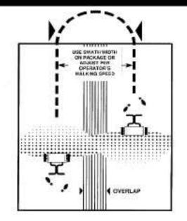
6. Push spreader at a normal walking speed -2 1/2 m.p.h. (18 feet in 5 seconds). Apply header strips around area to be treated. Space trips across the area as shown. Keep material off flower beds, sidewalks, etc.
