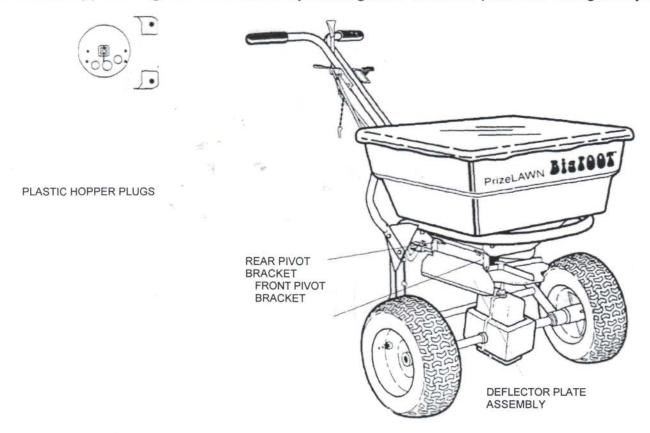
2. The deflector plate should be in the "DOWN' position as shown above. Insert the longer end of the control rod with the formed tab near the end of the rod into the universal bracket in deflector plate assembly as shown. Rotate the rod as shown to secure rod into the bracket.
