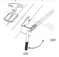
In the "ON" position, the material exiting the right hand side is deflected as shown. This allows the spreader to be butted up against a sidewalk, driveway, lot line etc. minimizing the amount of material thrown
