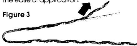
4) Insert the correct thimble size in the TREE-GRIP dead-end's cabled-loop and cross the longer leg with the already completed short leg at the cross-over mark. The thimble is now secured and cannot fall.
