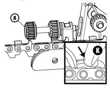
This forward movement corresponds to the quantity of material to be ground from the cutter. The more dull or damaged the cutters, the greater this forward movement should be. For cutters that are not too dull, simply grind a slight amount of material.
