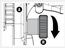
Rotate the entire motor unit (A) until the reference mark on the edge of the arm is positioned at the desired head tilt angle (11).
