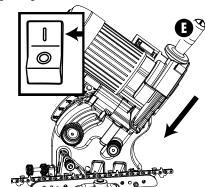
Once you have sharpened the first cutter, raise the motor unit with handle (E).
