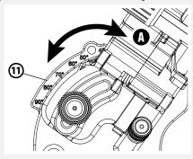
Tighten arm locking knob (H) at the back of the motor unit (A).
