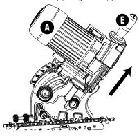
Turn the cutter adjustment knob (8) clockwise, to slightly move the cutter to be sharpened further forwards.
