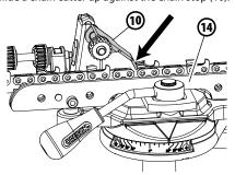
Turn the adjustment knob (9) to position the chain stop (10) laterally to the center of the cutter.
