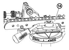
Slide a chain cutter up against the chain stop (10).
