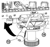
Advance the chain forward to position the next cutter to be sharpened, assuring that the chain stop (10) is seated firmly against the rear of the cutter.
