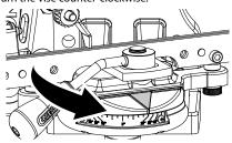
Position the reference mark pointer (17) on the vise by the desired vise rotate angle.
