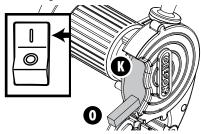
Stop the grinder by turning the switch to position "O".
