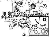
Set the depth gauge following the instructions given in the "OPERATING INSTRUCTIONS, SHARPENING THE CHAIN" section on pages 26–27 . For this type of sharpening procedure, there is no difference between the right and left cutters, therefore sharpen all the gauges one after the other.
