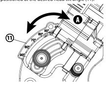
Tighten the locking knob (H) at the back of motor unit (A).
