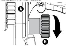
Rotate the entire motor unit (A) until the reference mark on the edge of the arm is positioned at the desired head tilt angle (11).
