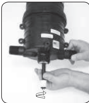
Step 2. Rotate #51 SHAFT 90° and pull from body.
