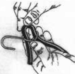
4. Thread rubber strap through other loop, leaving a tail to be wrapped back through.
