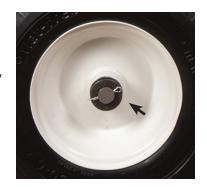
**STEP 4)** For pneumatic tire model #15CC, check for proper inflation as indicated on the tire and inflate as necessary.
