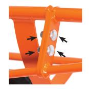
**STEP 2)** With cart frame laying front down on your work surface, slide the 3/4" axle rod through the frame axle housing leaving room on either side for wheel placement.
