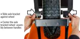
Slide axle bracket against wheel Center the axle
