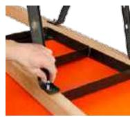
**Step 5)**Install Leg Brace -Keeping the #WB1002 Leg Brace to the inside of the Leg, line up holes in Brace and Legs, then secure using (4) 3/4" Square Shank Bolts, washers, and nylon lock nuts.
