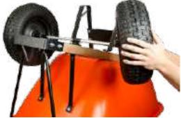
Secure Wheels - Install washer to outside of wheels, then insert cotter pin through axle hole and bend over with pliers.
