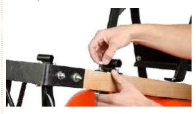
Front bolt secures both tray brace and axle bracket.
