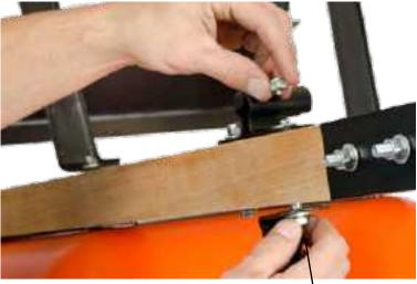
Front bolt secures both tray brace and axle bracket.
