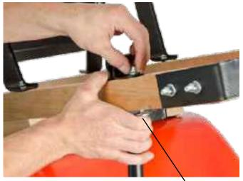
Front bolt secures both tray brace and axle bracket.
