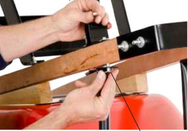
Front bolt secures both tray brace and axle bracket.
