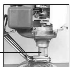
Picture 3... Note how the engine sits all the way down on the transmission.
