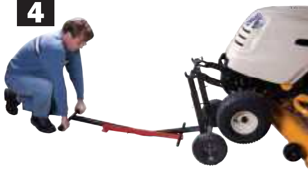
The tractor lift is securely in place when the curve in the handle is resting flat on the ground.
